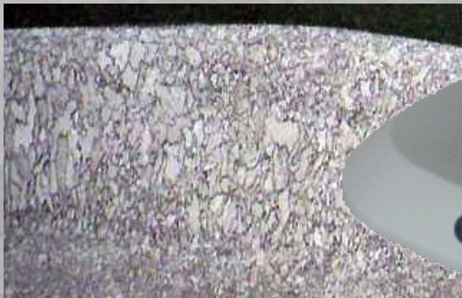
Stereo microscope image of filler metal in a steel weld
