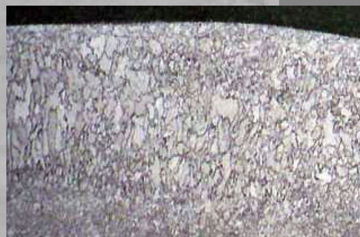
Stereo microscope image of filler metal in a steel weld
