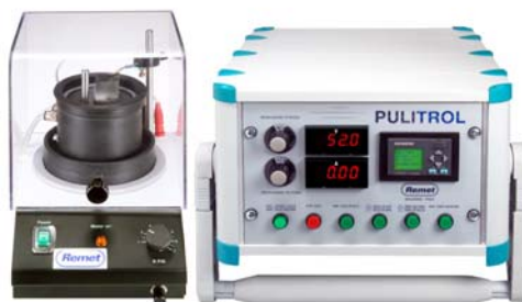
Figure 7-2 Electropolisher cell and control unit (Photo courtesy of Remet Italy).
