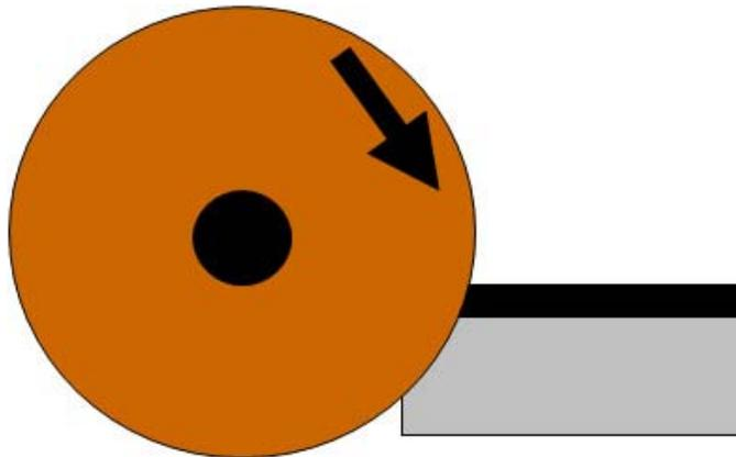
**Figure 2-3** For coated samples, maintain the coating in compression when sectioning.
