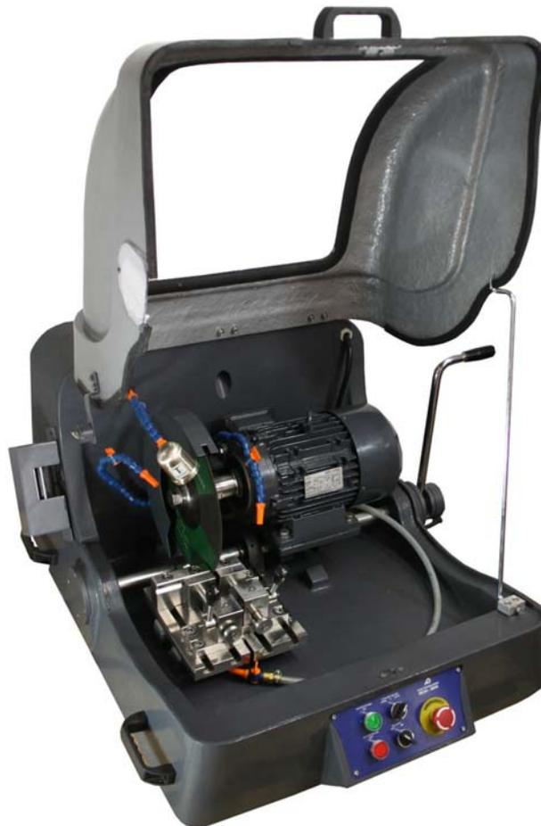
**Figure 2-5** MEGA-M300 Manual Abrasive Saw.
