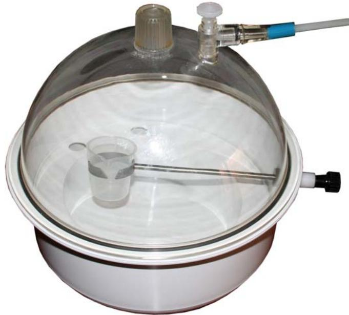
**Figure 4-5** Vacuum impregnation device.
