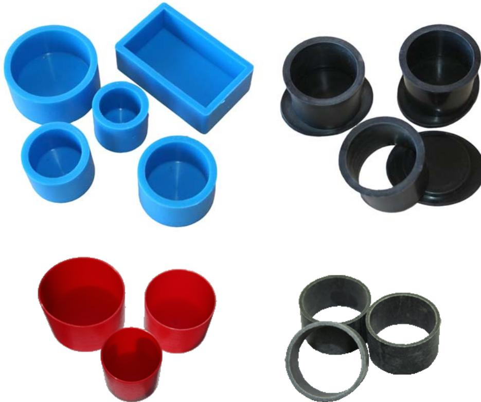
**Figure 4-6** Castable mounting molds
