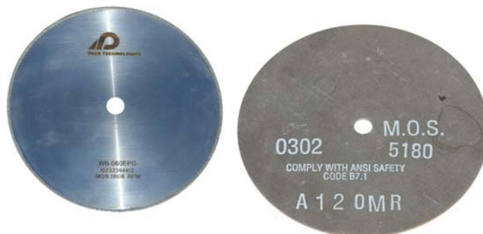
Figure 3-3 (a) Electroplated diamond wafering blade for cutting soft materials (left) and (b) alumina resin-rubber blade (right).
